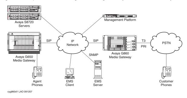
Figure 59: Sample call center configuration using the Avaya G860 Media Gateway
